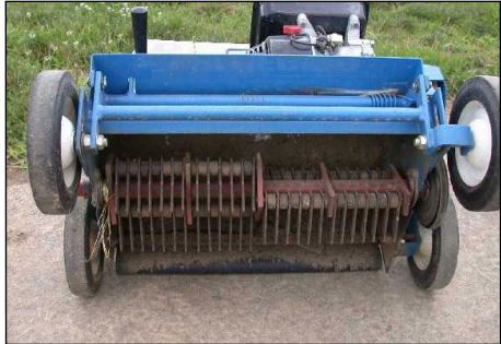
Power rakes should be set to slice through the top ½ inch of soil to create a seedbed.
