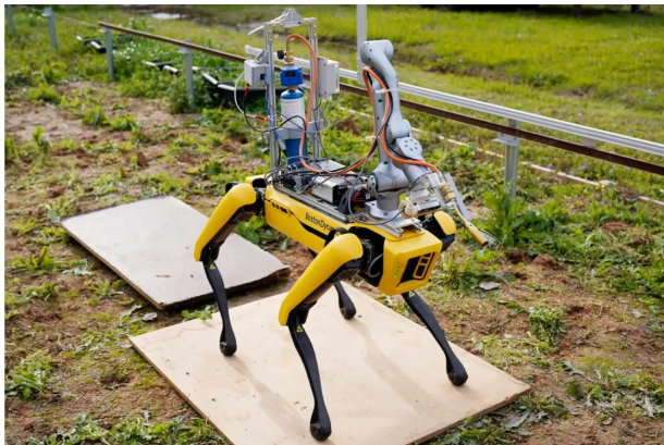
▲ A Spot robot equipped with a blowtorch for tackling weeds Dezhen Song et al. (2024)
