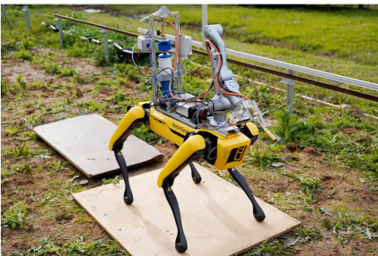
★ A Spot robot equipped with a blowtorch for tackling weeds (Dechen Song et al. (2024))
