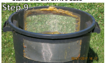
Step 9 Both steel mesh windows in place
