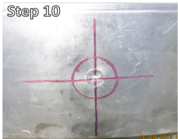
Step 10 At the center of the lid, draw an "X" that is 4 inches by 4 inches. Draw a 2 inch circle around the center.
