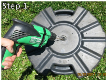
Step 1 Drill small holes in bottom of the 32 gallon bin with 3/8ths inch bit to allow rain water to drain.
