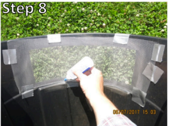
Step 8 Lay the bin on one side and secure the aluminum screen inside with duct tape. Glue the screen to the bin and allow glue to dry overnight. Gorilla glue is best—you can also use epoxy or E6000.
