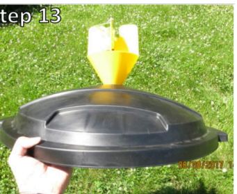
Step 13 Push the base of yellow commercial top through the slots you made.
