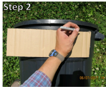
Step 2 Cut a 5 by 15 inch rectangle out of cardboard. Use as a template to draw 2 windows (one on each side of bin)
