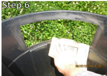
Step 6 Use sandpaper to sand the inside edges of the windows. This will allow the glue to adhere to the plastic. WARNING: Do not use hot glue because it will melt outside in the summer heat!
