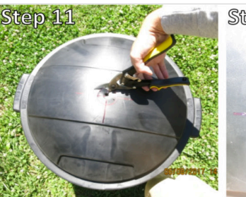
Step 11 Drill a large hole in the center and use that as a starting point to cut out the "X" & circle shape you drew.
