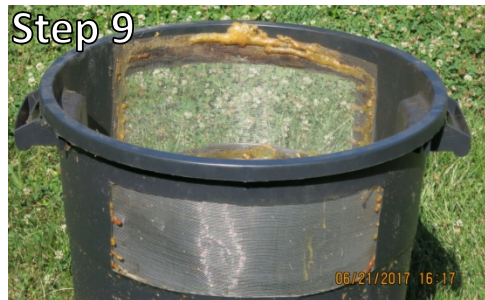
Step 9 Both steel mesh windows in place
