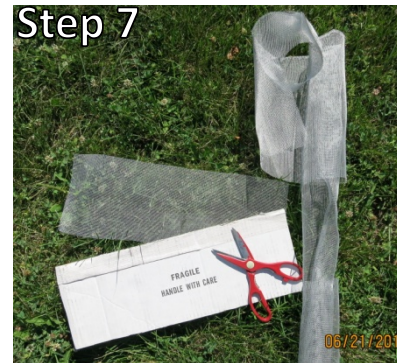
Step 7 Cut a 7 by 20 inch rectangle out of cardboard. Use this template to cut out 2 window screens.
