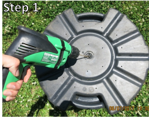
Step 1 Drill small holes in bottom of the 32 gallon bin with 3/8ths inch bit to allow rain water to drain.
