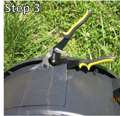
Step 3 Use an aviation "tin-snip" tool to cut out the window you traced with permanent marker.
